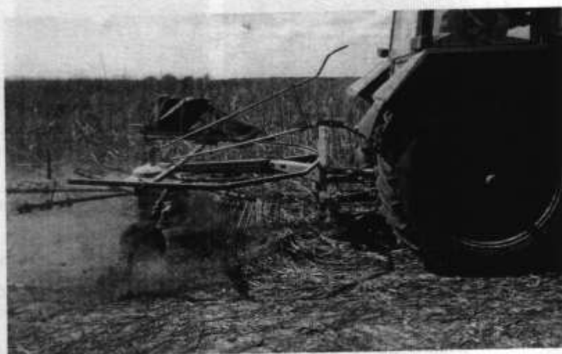
Fig. 6. Use of rotary rakes when harvesting hemp stems
